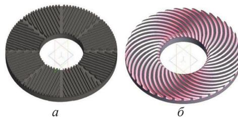
Fig. 2. The schemes of the knife tackings: *a* – with rectilinear knives; *b* – with curvilinear crescent-shaped knives
