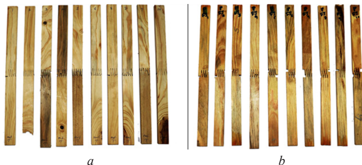
Fig. 4. The untreated (a) and treated (b) failure finger-jointed samples
