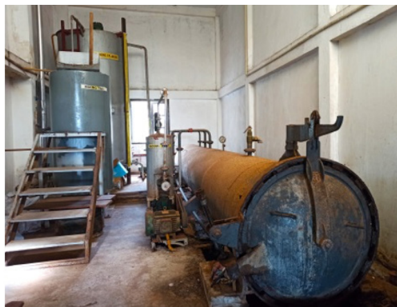
Fig. 1. The vacuum pressure impregnation plant
