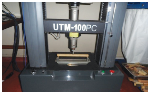
Fig. 2. The Universal testing machine (UTM-100PC)
