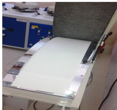
Fig. 3. Drying the sheet by means of a temperature controlled laboratory dryer
