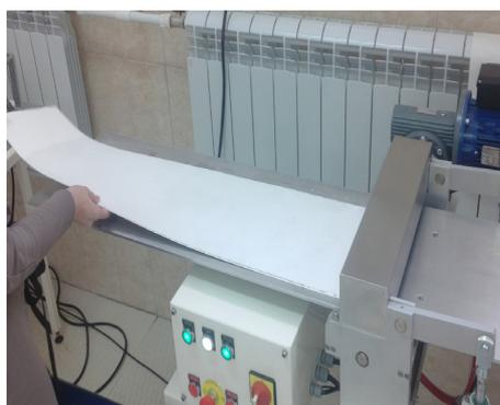
Fig. 2. Pressing the handsheet by means of a pneumatic single-drum press
